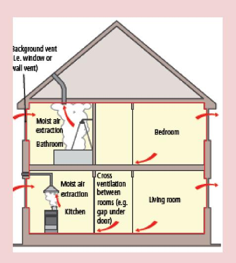
Ventilation in the home using a combination of mechanical vents and natural ventilation
